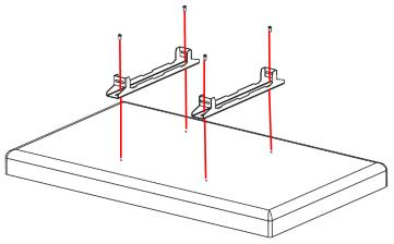
Carefully lower the screen onto the mount and secure in place using an M6 bolt on each side of both hangers.
