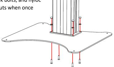
Secure the mount to the headbox using four M8 bolts.
