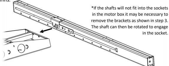
3. Gently remove the transportation brackets from columns as shown, put the bolts removed to aside for use later in the assembly process.
