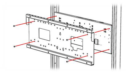
13. Attach the hangers to the back of the screen.
