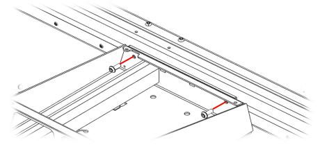
5. Plug the power cable into the transformer though the grommet indicated and bolt the rear panel in place.
